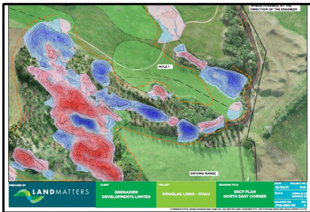
Fig 4: Proposed Earthworks to establish building platforms at the centre of the site
